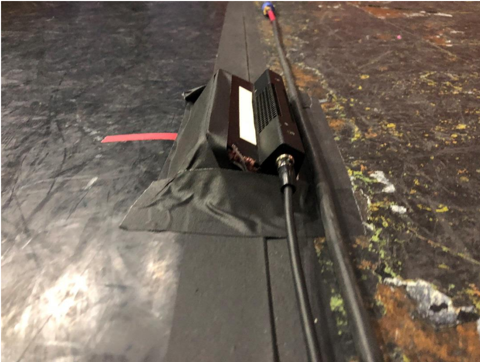
Positioning of PCC mics for best pick up (side view)
